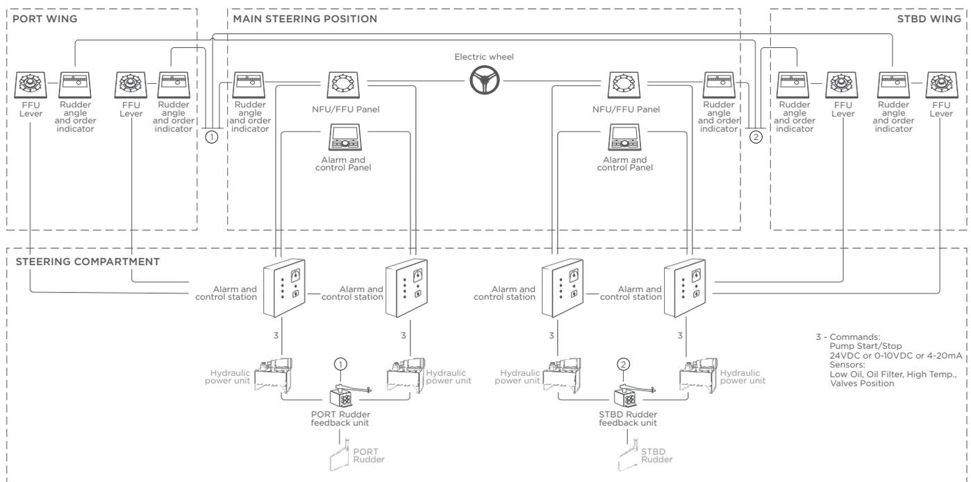
In the figure: two independent steering gears with two pumps in each gear is completely processed by represented STCS5000 system on three steering positions.
